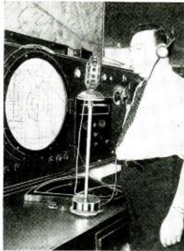
Dr. S. Spitz, of Burbank, Calif., developed this amazing machine, which indicates as a moving spot of light, the location of an airplane; the 'plane's sound automatically actuates the device. The same principle probably could be applied to silent 'planes, the actuation then being obtained by means of centimeter (the "mystery ray" mentioned in this article) waves reflected from the 'plane!
