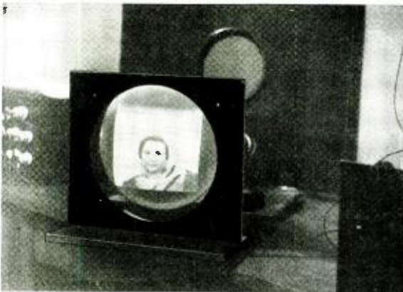
Untouched Television view—reproduced by a Von Ardenne cathode-ray scanner. Remarkable grain and line structure are indicated.
